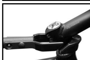
Extend the bar until the large hook can be placed around the stem and close the lock.
