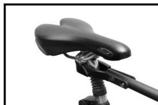
Place the small hook around the seat post and close the lock.
